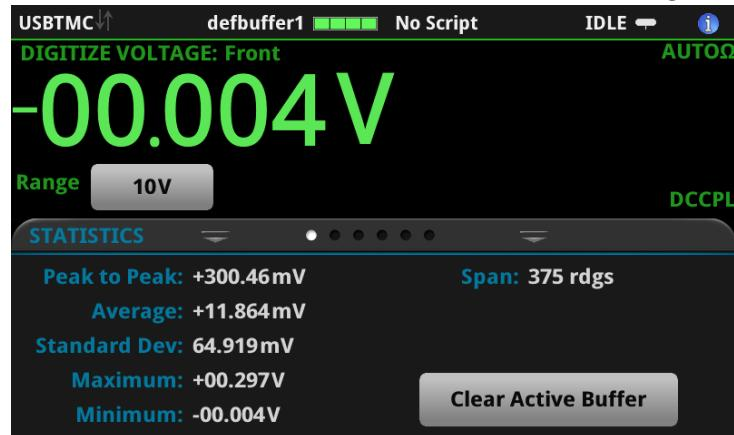
Use that maximum voltage as a hint to a peak detector algorithm written in the Lua based TSP scripting.
